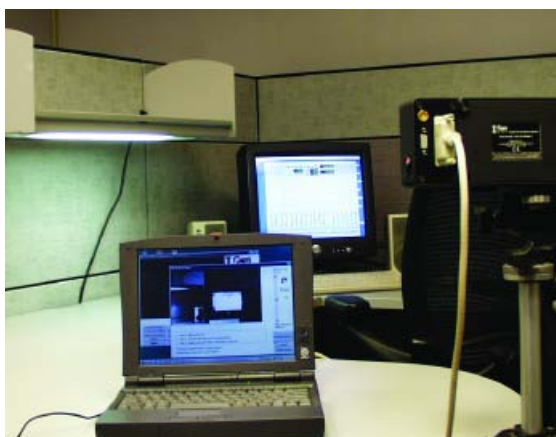
Figure 9 — Visibility Testing of Workstation — Video Photometry
